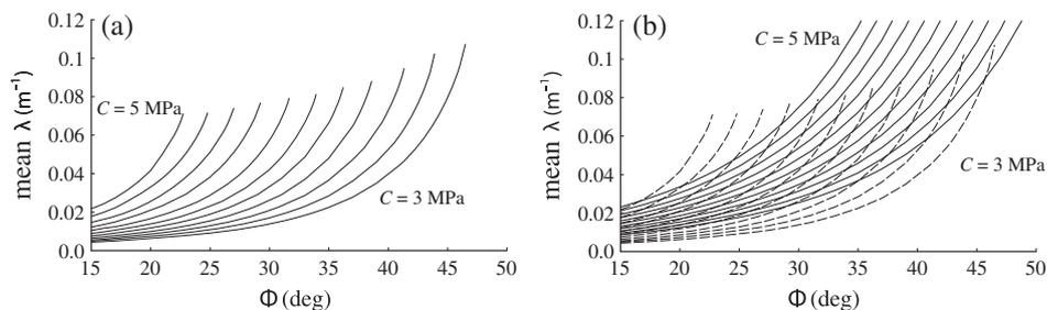
Figure 10. Mean value of erosion strength  $\lambda$  for the cases (a)  $\sigma_{\text{out}}=7.5$  MPa and (b) 11 MPa. The curves are labelled by the values of the cohesion  $C$  in range 3–5 MPa differing by 0.2 MPa. The curves of the case (a) are also plotted in dashed line for comparison with the case (b).
