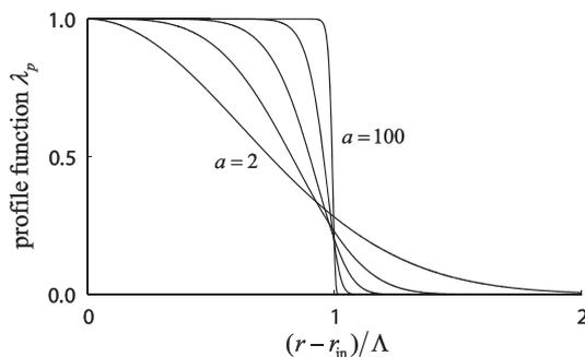
Figure 2. The erosion profile function  $\lambda_p$  for  $a=2, 4, 8, 20, 100$ .
