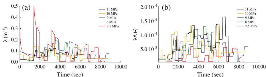
Figure 9. Behaviour of (a) erosion strength and (b) product of erosion strength with plastic zone depth with respect to time.
