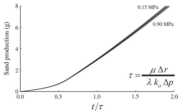
Figure 7. Predicted sand production curves for external stress 11 MPa and the different pressure drop level (different flow rate) in scaled time. The curves are practically self-similar.
