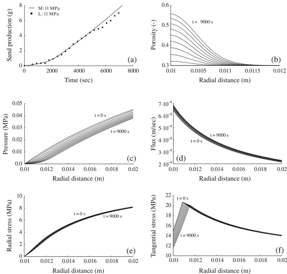
Figure 6. Sand production hydro-mechanical solution according to the proposed model for external stress level 11 MPa and pressure drop 0.15 MPa: (a) cumulative sand production, (b) porosity profiles, (c) pore pressure profiles, (d) fluid flux profiles along the hollow cylinder, (e) radial stress profiles and (f) tangential stress profiles from time 0 to 9000 s for every 1000-s interval.
