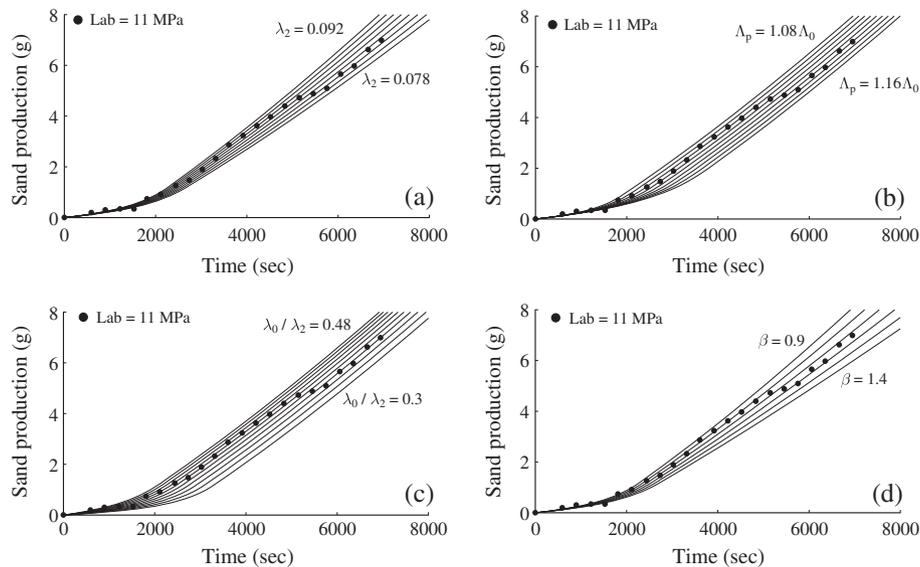
Figure 8. Influence of model parameters on the shape of the sand production curve with external stress level 11 MPa and pressure drop 0.15 MPa: (a) maximum erosion strength  $\lambda_2$ , (b) threshold depth  $\Lambda_p$ , (c) ratio of initial to maximum erosion strength  $\lambda_0/\lambda_2$  and (d) model exponent coefficient  $\beta$ .
