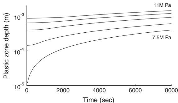
Figure 5. Progression of the plastic region depth  $\Lambda$  as predicted by the model for the cases of 7.5, 8, 9, 10 and 11-MPa external radial stresses.
