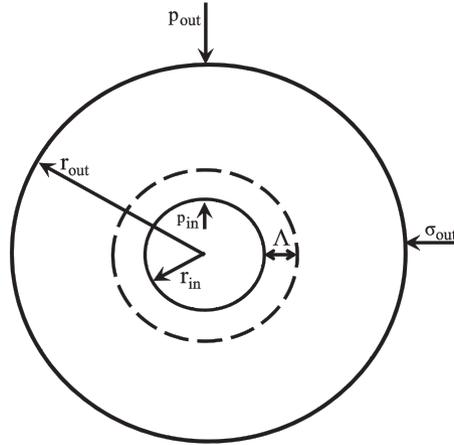
Figure 1. Schematic of the hollow cylinder problem to simulate the erosion process under radial flow.
