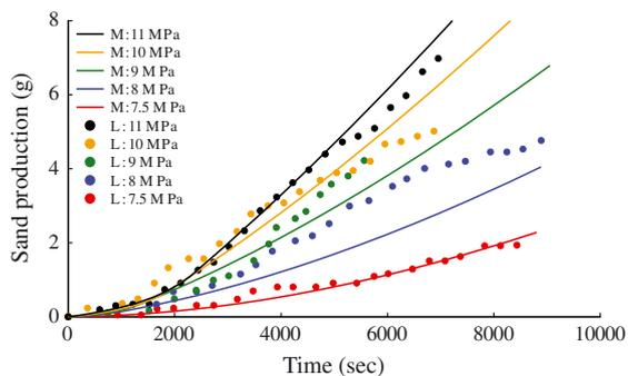
Figure 4. Comparison between the curves predicted by the model (denoted as ‘M’ - continuous lines) with the test data of Papamichos *et al.* [13] (denoted as ‘L’ – marker points) for fixed pressure drop  $\Delta p=0.15$  MPa (flow rate  $Q=0.5$  l/min).
